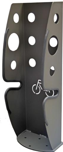
PDL MS is a new bike rack to park two cycles (in the same direction) on public areas and community spaces that takes up very little space. The cycle is set through the introduction of the pedal in the aperture and keeps stable. The user must bring the padlock to lock a rear wheel and the frame.
